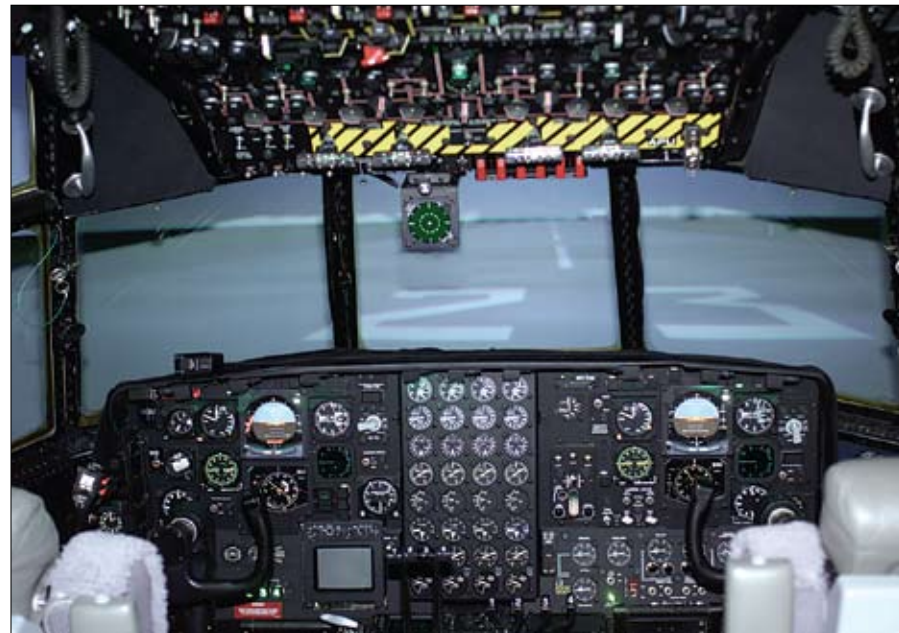
KC-130T APT developed and manufactured at the J.F. Taylor, Inc. facility from a salvaged cockpit shell.
