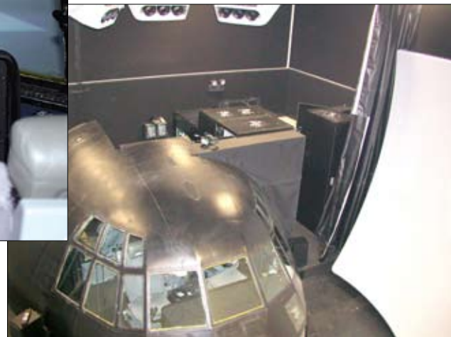
KC-130T APT developed and manufactured at the J.F. Taylor, Inc. facility from a salvaged cockpit shell.
