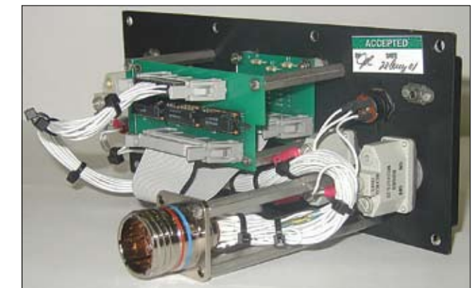
Fuel management panel, back; front is shown below left.
